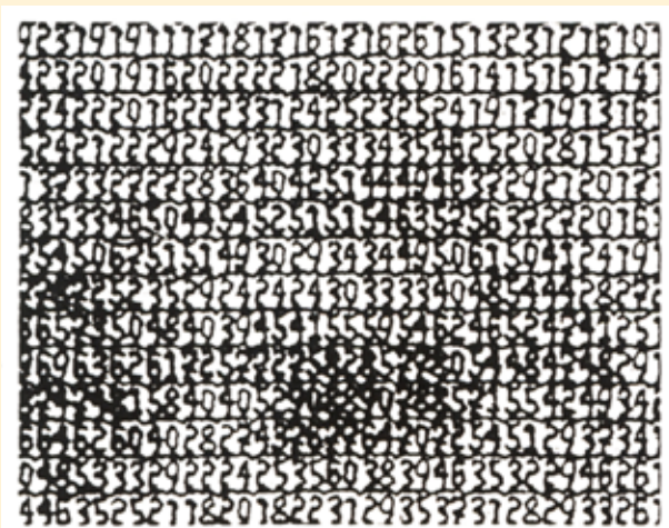
Figure 1 — This shows a close-up of one of the eyes of the digital Mona Lisa. Here the decimal digits in the cells can be seen; the digits are not visible in the reduced, screened picture on the front cover.
